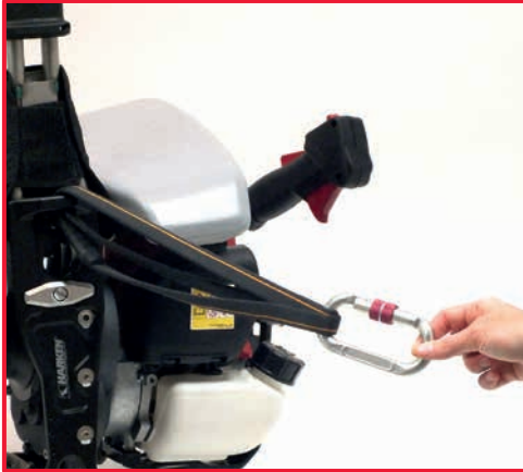
Check that the stop and carabiner are intact.
