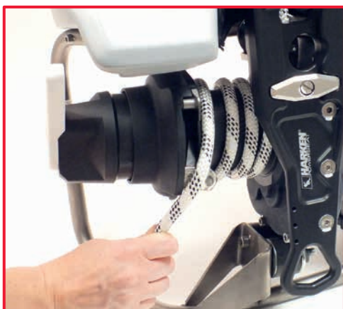
8. Pass the rope over the stripper arm.
