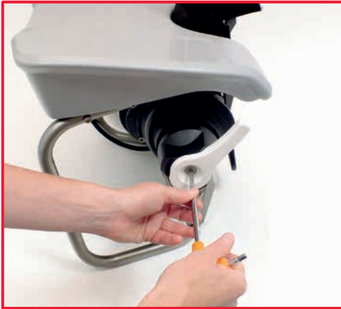
1. Loose the control lever screw.
