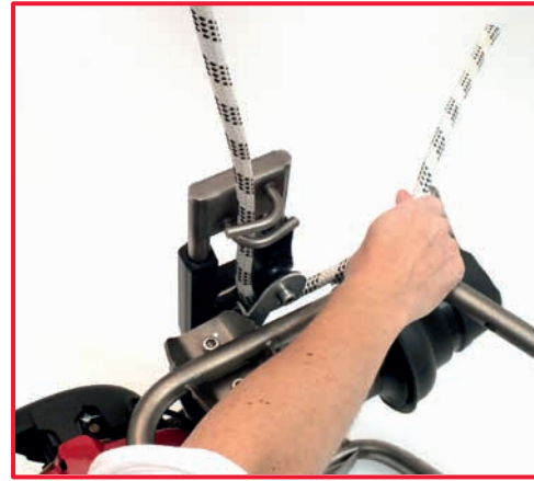
6. Pass the rope round the pulley.
