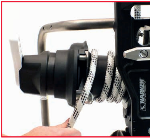
9. Pass the rope over the stripper arm.
